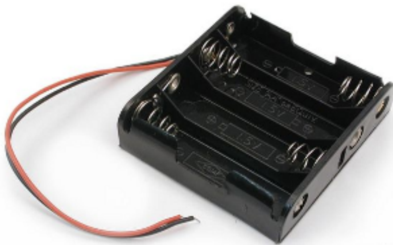
FIGURE 2. – Support de pile AA
